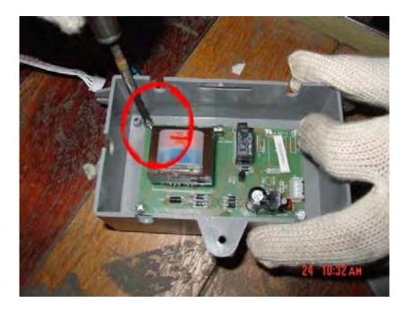
8. Connect the terminal on the control board.
