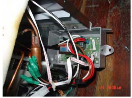
5. Disconnect the terminal on the control board.
