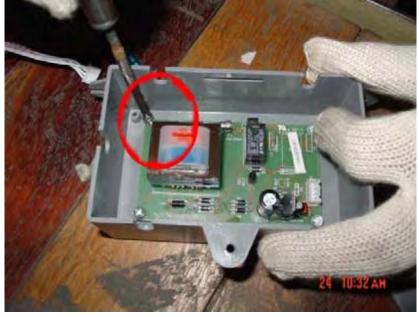
7. Replace the control board with a new one and fasten the screws.
