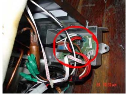
9. Place the control board cover back into position and fasten it with the screws.
