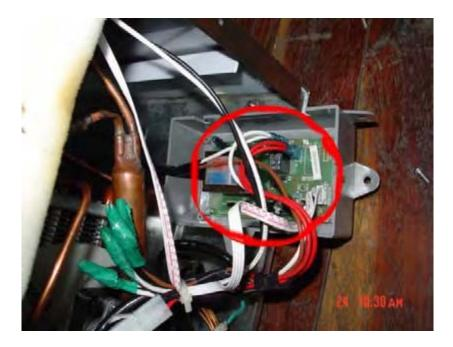
6. Remove the screws from the control board.
